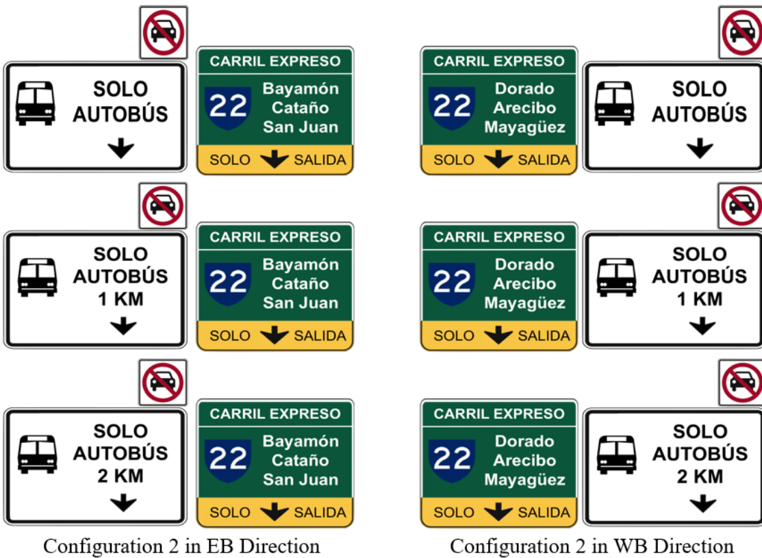
Figure 3.2 Configuration 1 and Configuration 2 signs in each direction.
